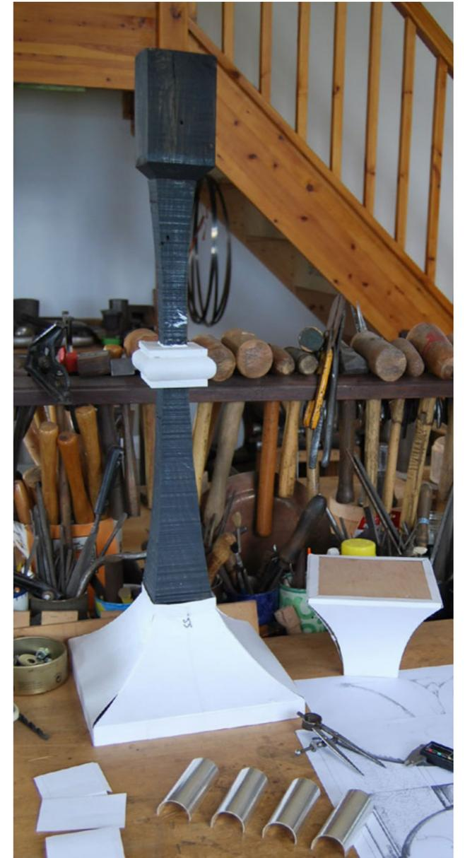
Model for the altar candlesticks with four half-round silver tubes as part of the construction of the knob
