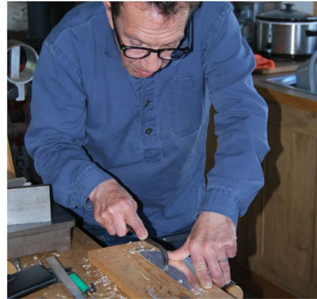
Kelly scoring the silver with a sharpened cutter. The silver can then be folded along the score to produce the right profile
