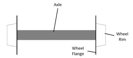
The wheels are made from steel and have flanges on their inner edges. It is sometimes thought that the flanges are necessary for the wheelset to follow a curved track. However, this is not the case: the wheelset would follow a curved track even without the flanges.
